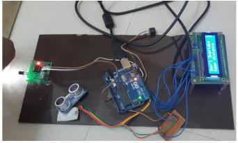
Figure 2.2: Buzzer sounding in case of fire emergency
