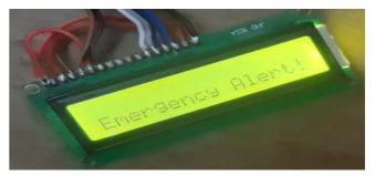
Figure 2.5: LCD display of an emergency
