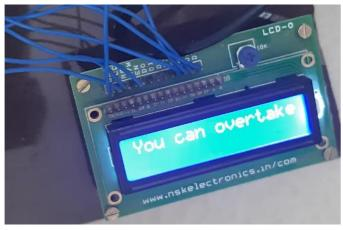
Figure 2.3: LCD display to overtake
